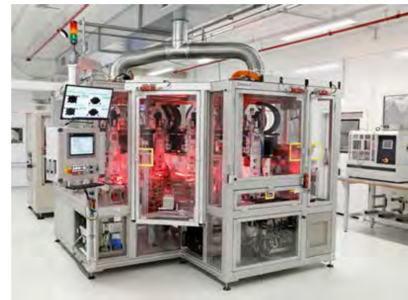
An automatic handling machine stacks electrode sheets
